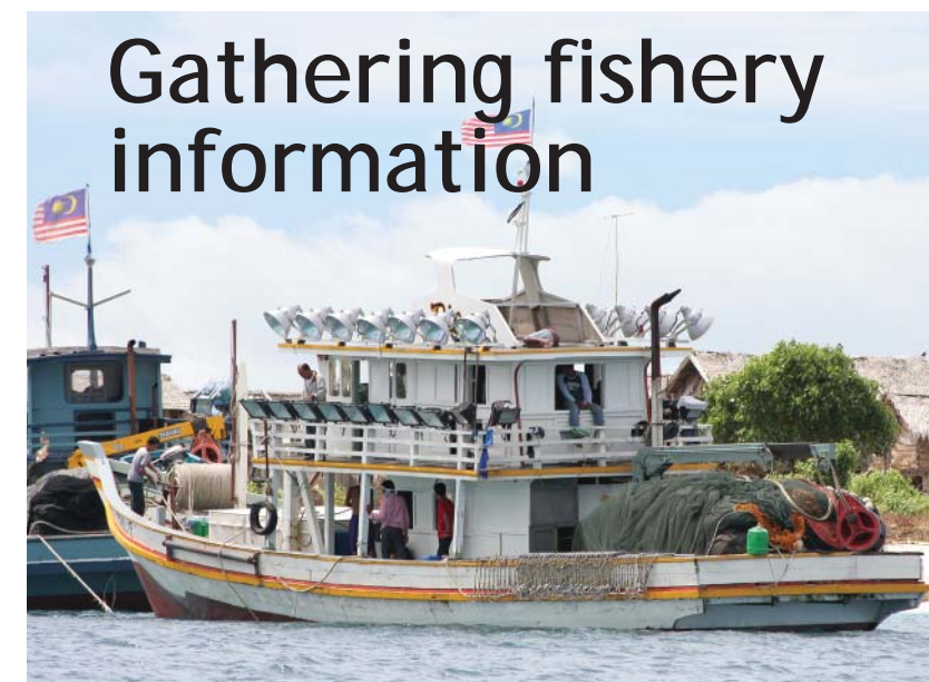
This boat hauled up on Pulau Maiga operates at night, using a purse seine (encircling net) to capture pelagic species such as tuna, mackerel, sardines and scads.
